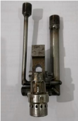
图 2 某型航空发动机离心式雾化喷嘴 Fig.2 Centrifugal atomizing nozzle for an aero-engine
